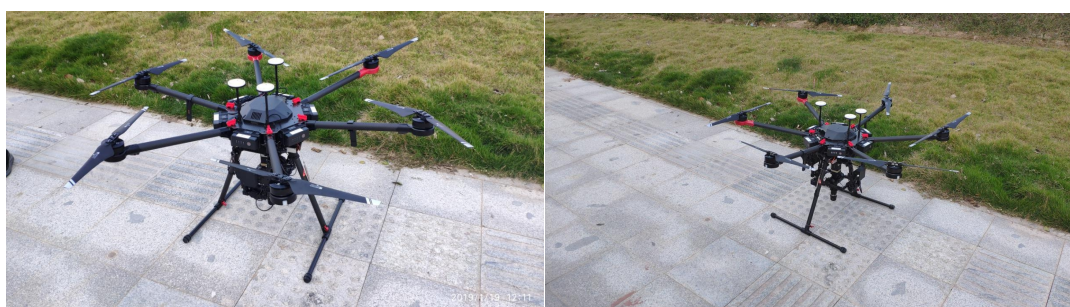
Fig 13 Left: ATH1500 VIS-NIR hyperspectral imaging camera; right: ATH1500-17 SWIR hyperspectral imaging camera
